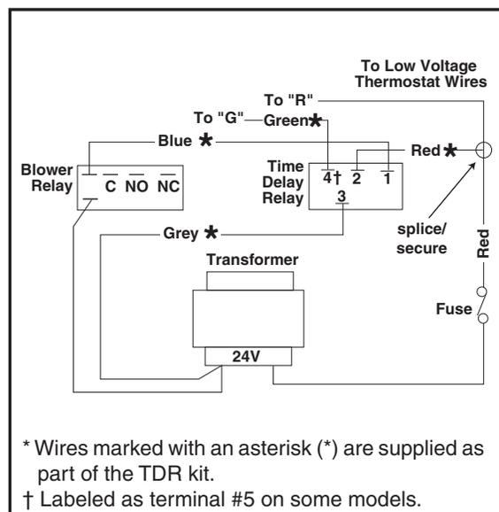
**Figure 3. Wiring Diagram for E(1,2,3)EB Electric Furnace Applications.**
